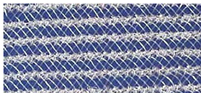
Translucent monofilament fibre exclusion netting with heavy weave (2 mm)
