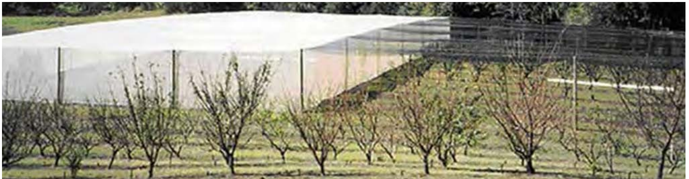
The fruit fly (LHS) and bat (RHS) exclusion netting trial at Maroochy Research Station
