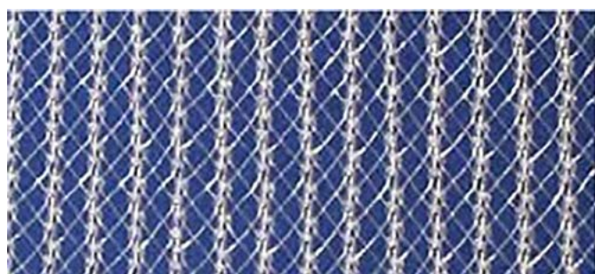
Translucent monofilament fibre exclusion netting with light-weave (2 mm)
